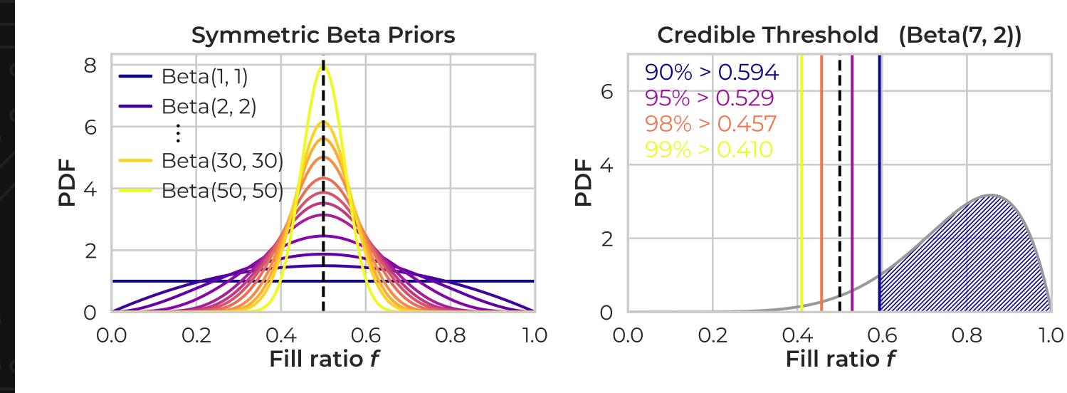
• Robots making *fewer* observations improves accuracy by reducing spatial effects • Selecting a sufficient regularizing prior allow for a lower credible threshold with a
