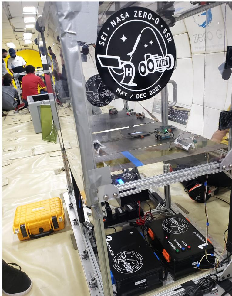
**Figure 7.10:** Experimental box for Zero-G flight testing. The walking Ferrobot is located on the nearest plate and tethered to control boxes placed underneath the frame. (Image courtesy of Bahar Haghighat.)
